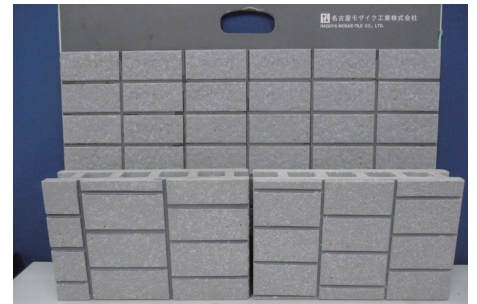
Comparison of ceramic tiles(top)and a KEPT sample(bottom)
